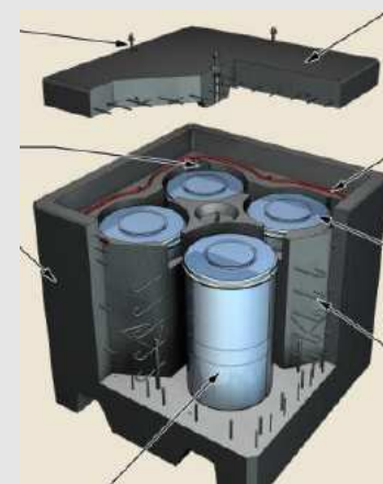
Conteneur de stockage, image ANDRA
